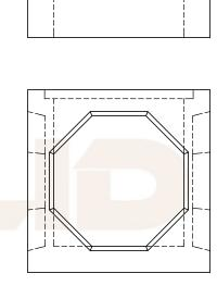
Concrete 28 day compressive strength of 4,500 PSI Bottoms to be monolithic at floor and at first stage of wall
