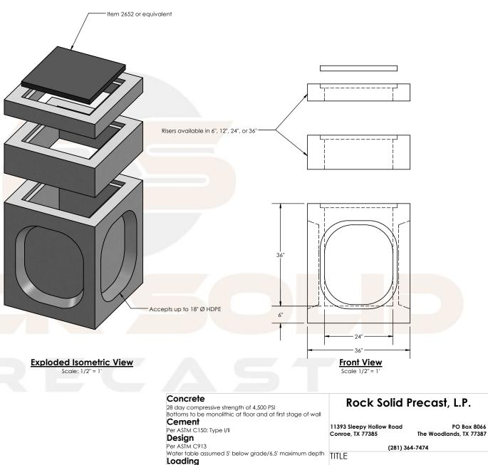
Rated for HS-20 Cast Iron Meets ASTM A48 and CL35B Standards
